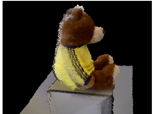
Figure 8: Predicted surface generated from freiburg1_teddy dataset. Reconstruction of the dataset after 300 frames.
